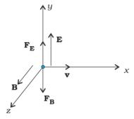
Consider a point charge, q moving with a velocity, v in a direction perpendicular to both mutually perpendicular uniform electric and magnetic fields as shown in the diagram.
