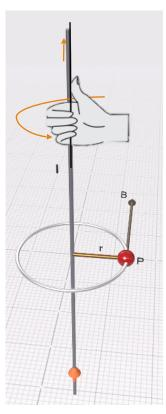
Consider an infinite straight conductor carrying current I. Let P be a point at a perpendicular distance r from the conductor. In this case the amperian loop can be an imaginary circle with conductor as is perpendicular axis and P on its circumference.
