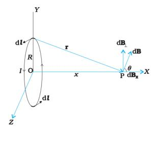
coil at a distance of x from the centre O. Let dl be a current element of the coil as shown which is distant r from P.
