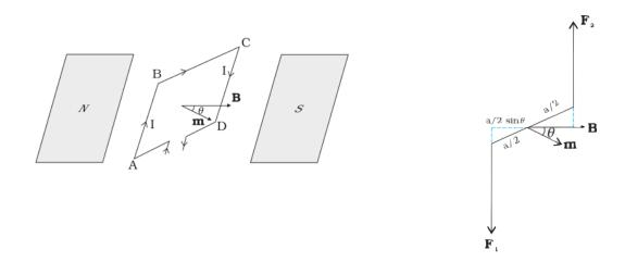
Let the angle between the field B and normal to the coil is  $\theta$ .
